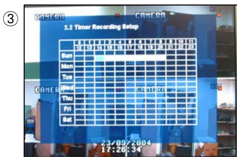
After 'Deselect' Schedule, Activated Region by Press 'ENTER' and Select Date & Time to Move Cursor
